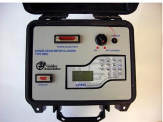
The SM02 SGMETER is designed to read and record data automatically from multiple single arm strain gauges, as used in Golder RMT's instrumented rock bolts. Its rugged construction makes it ideal for use in the mining and civil engineering industries.
